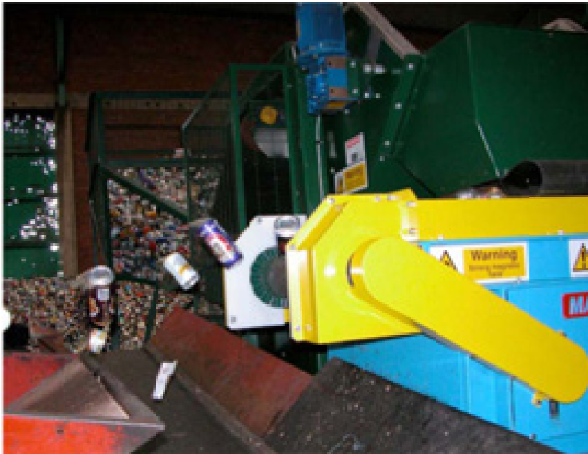
Figure 4-11 Illustration of an eddy current separator
